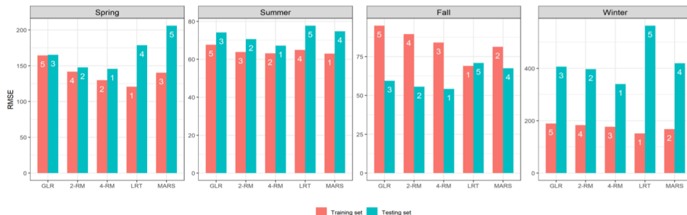
Fig 2: Mean squared errors (MSE) for PM_{2.5} on the training (red) and testing (green) sets for each season of five models, including global linear regression (GLR), two-regime model (2-REG), four-regime model (4-REG), linear regression tree (LRT) and multivariate adaptive regression splines (MARS), with model ranks (in increasing order of the MSEs) marked on top of the bars.
